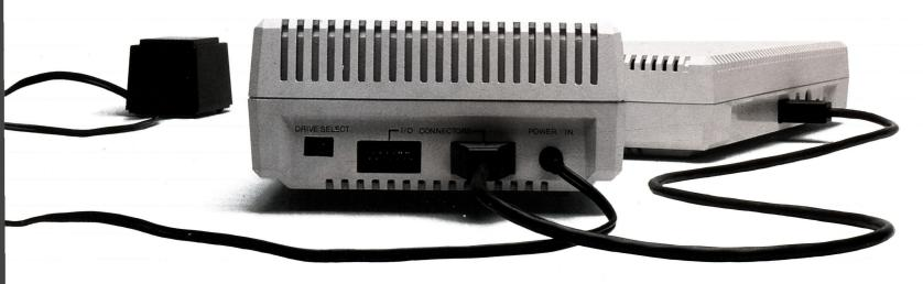
As many as four disk drives, in addition to other components, can be connected to the ATARI Home Computer by Serial I/O Cables supplied with components. To install multiple drives, connect a cable between one I/O CONNECTOR jack on the first drive and a PERIPHERAL jack on the computer console. Connect another cable between the remaining I/O CONNECTOR jack on the first drive and an I/O CON-NECTOR jack on the second drive. Connect additional components in the same manner.
