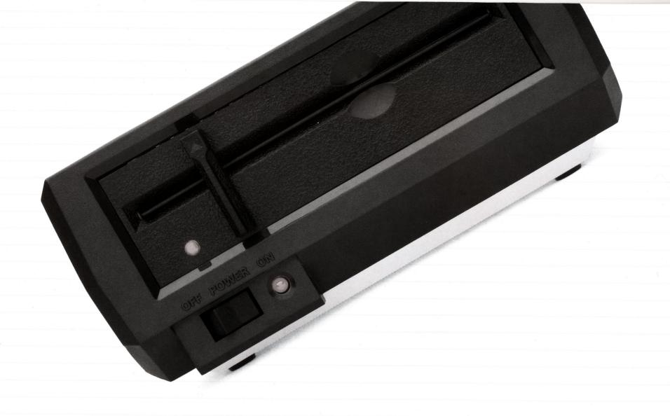
n extremely efficient high-speed memory device, the ATARI 1050 Disk Drive greatly enhances the capabilities of your ATARI Home Computer. You can store and manage large quantities of information in separate files on floppy diskettes. You can retrieve files by name, copy or erase them, and manage them in other useful ways.
