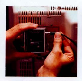
Locate the round cord that comes from the back of computer console. Plug the end of this cord into the terminal on the TV ritch Box labeled **Computer** or **Came**. Make sure the TV Switch Box is set to the **Computer** position.
