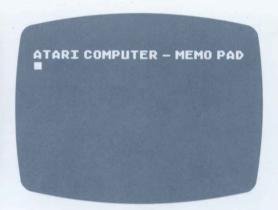
You're now ready to turn on your computer. The main power switch, labeled Power On/Off, is located on the side panel. As soon as you turn it on (provided the cartridge door is closed and no cartridge is inserted), the words ATARI COMPUTER – MEMO PAD appear on your TV screen. Whatever you type on the keyboard is now displayed on the TV screen.
