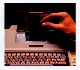
Insert the cartridge into the slot with the label facing you. Press down carefully and firmly. When you close the cartridge door, the red power indicator at the right of the keyboard lights up, and the TV screen displays the title screen for the cartridge you selected. Then follow the instructions that come with the cartridge.
