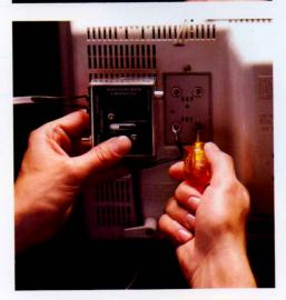
Now locate the short twin-lead cable marked **TV** that comes from the TV Switch Box and connect it to the two VHF terminals on your TV set.
