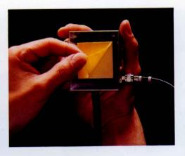
Peel off the protective cover sheet from the self-adhesive square and stick the box onto the back of your TV. If your TV set was connected to a flat, twin-lead (300 Ohm) cable, you're finished installing the TV Switch Box.
