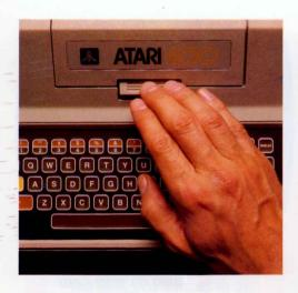
ush the cartridge door release lever down to raise the cartridge door. Whenever you do this, the ATARI 400 computer automatically turns itself off. It turns itself back on when you close the door.
